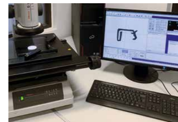
Profile cross-section inspection of a radial shaft seal
