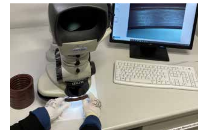
Surface inspection of a radial shaft seal using an electronic microscope
