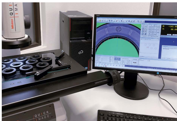
Dimensional inspection of a radial shaft seal using a measuring microscope
