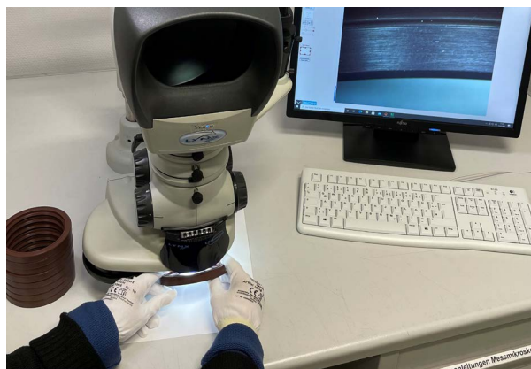
Surface inspection of a radial shaft seal using an electronic microscope
