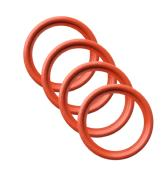
Metal-detectable O-rings are like a traditional elastomer seal with adding metallic fillers that allow metal detectors to quickly identify and find contaminated products. When any seal is subjected to excessive use or continuous use in demanding application damage can occur causing the seal to degrade increasing the risk of fragments of the elastomer ending up in the product being manufactured.
