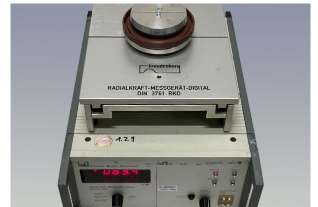
Radial force measurement of a radial shaft seal
