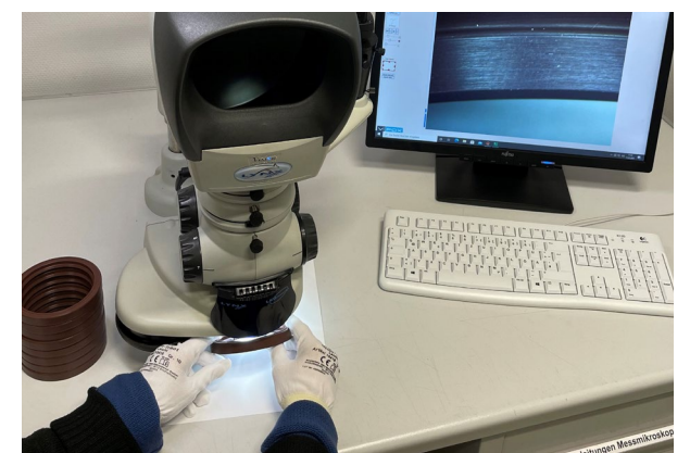
Surface inspection of a radial shaft seal using an electronic microscope
